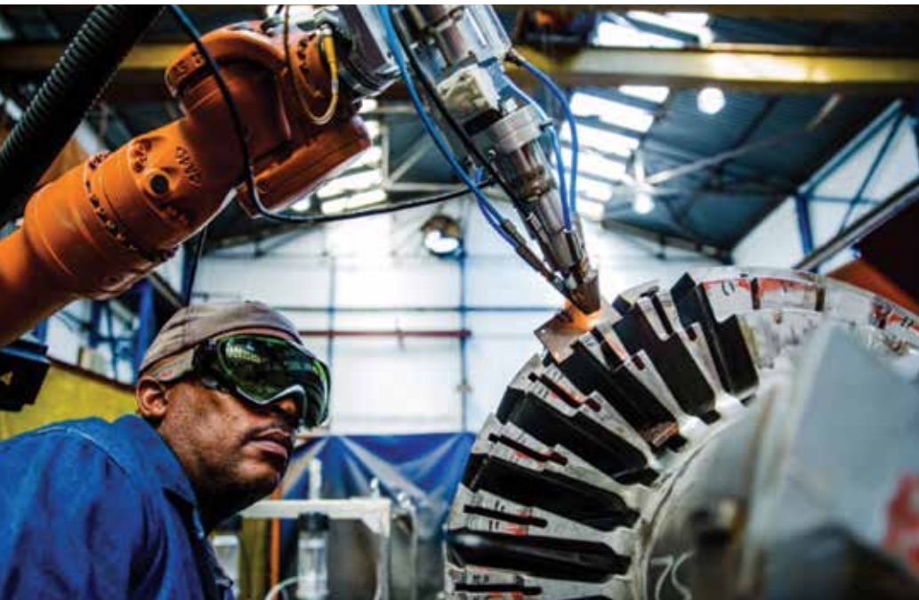
"A technician observes the laser refurbishment of a generator rotor" by Pieter Uys
