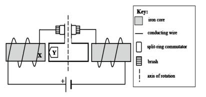
What is the polarity of the electromagnet at **X** and the direction of motion of the wire at **Y**?
