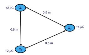
What will the magnitude and direction of the resultant electrostatic force on Q<sub>3</sub> be?
