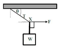
Which one of the following diagrams is the correct force triangle for this system?
